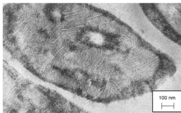
Figure 12 TEM images obtained on sections from PP/EP18 (upper) and PP/EP15 (lower) samples.
